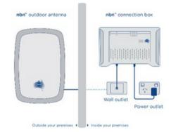
This technology is widely utilized in rural areas or when alternative options are not feasible. An external antenna is linked to the NTD using fiber optic connectivity, located within the premises as depicted in the image. Utelecom is responsible for delivering the service up to the NTD and supplying and maintaining the router if provided. The customer assumes responsibility for connecting their devices and managing the cables within the premises, although basic support is available.
